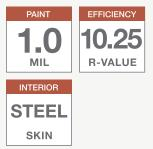
2" thick insulated steel sandwich panel constructed of top quality materials. Highly detailed raised ranch panel, deep woodgrain texture, and two coat prefinished paint system all combine to enhance the beauty of your home.
